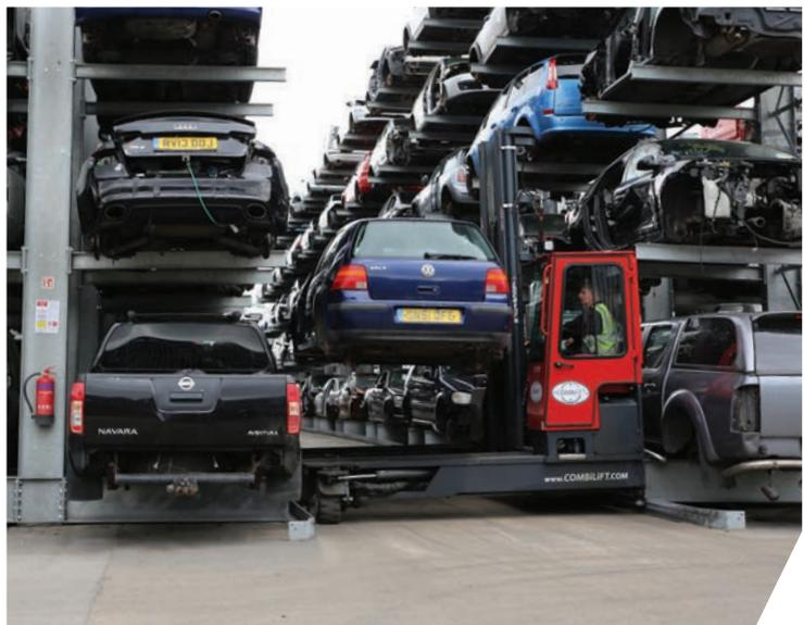
ASM contacted Locators Storage Systems to make a proposal for a cantilever racking system to maximise the storage capacity of vehicles awaiting processing. Previously, ASM had used counterbalance forklifts to move vehicles on other sites, but the aisle width required for counterbalance truck operation does reduce overall site capacity.
