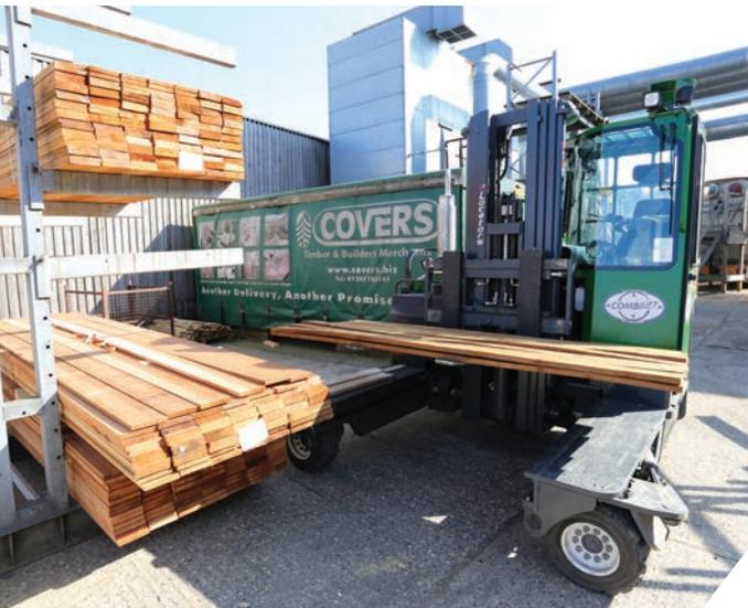
Locators has looked at each application on its own merit and proposed the right Combilift 4 way machine for the job. The electric trucks are able to work both inside and outside and Combilift trucks now carry out the work of the traditional sideloaders and reach trucks Covers had been operating.
